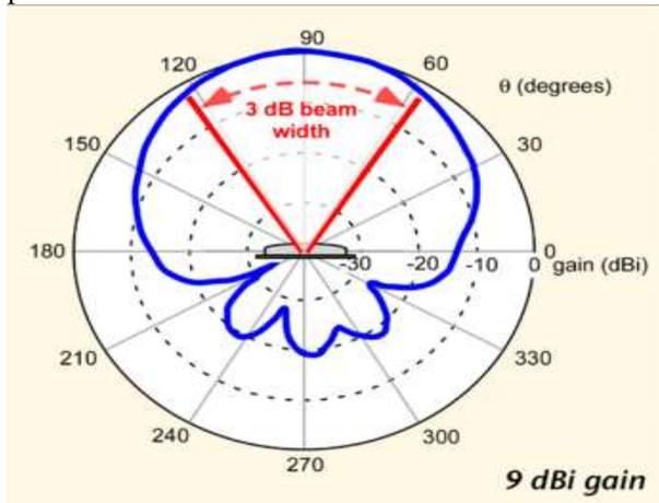
Fig. 5: Radiation pattern of antenna
