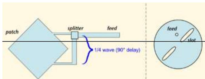
Fig. 3: Patch antenna design
