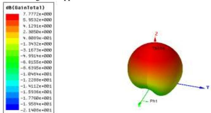
Fig. 9: 3D polar plot of antenna
