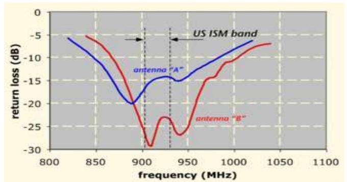
Fig. 8: Return loss of antenna
