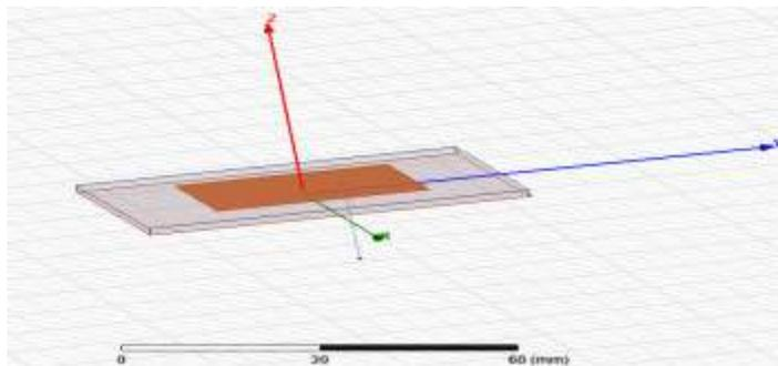
Fig. 1: Rectangular patch antenna
