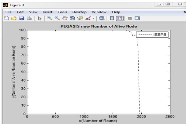
Fig 5.2 PEGASIS based graph between No.of alive nodes and rounds
