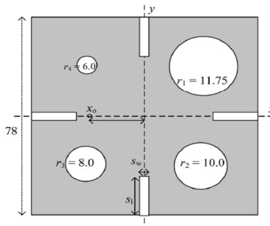
Fig. 2. Asymmetric- circular shaped slotted microstrip patch radiator. [2]
