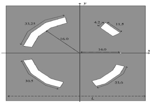
Fig3. Arc-shaped slotted square patch. [3]
