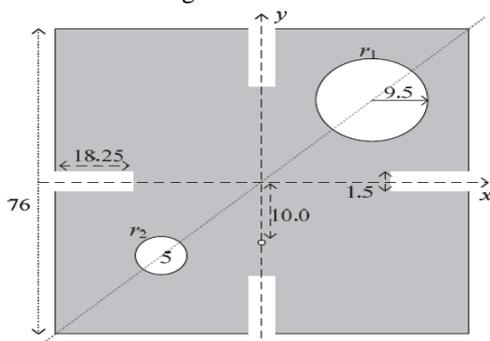
Fig4. Slotted-slit-microstrip patch radiator. [4]
