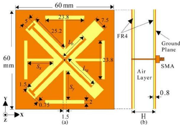
Fig. 6. Geometry of X-shaped slotted patch antenna. [6]
