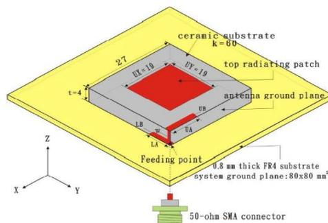
Fig5.3-D view of antenna. [5]
