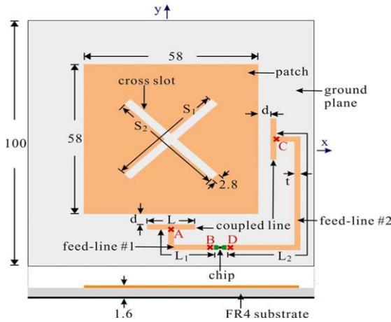
Fig. 4 CP RFID Tag Antenna [3]
