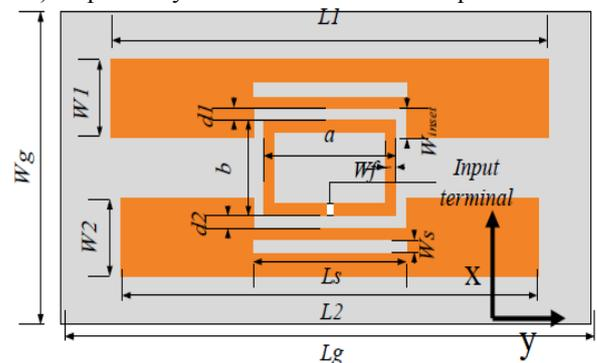
Fig. 6 Wideband Patch Antenna with Two C-shaped Patches [5]
