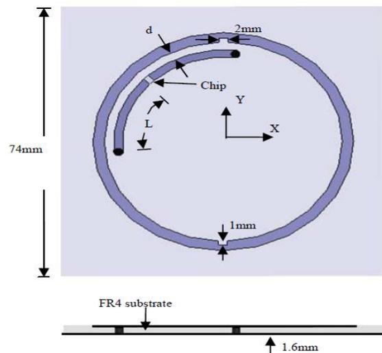
Fig. 8 Novel Design of tag antenna with annular-ring patch [7]
