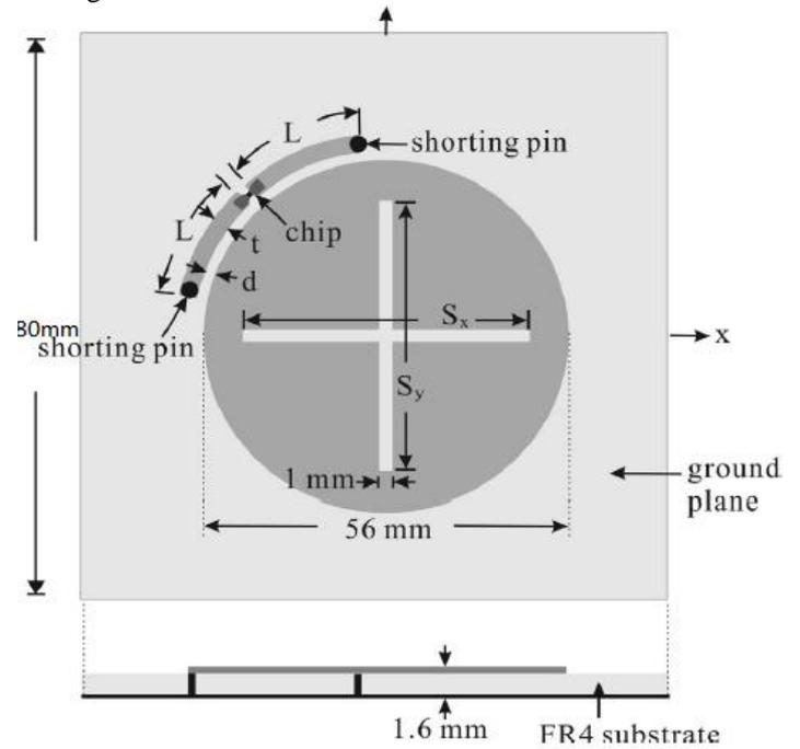
Fig. 5 CP Circular Patch Antenna [4]
