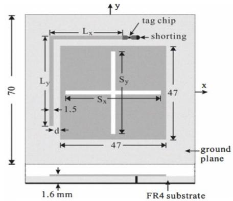
Fig. 2 Square Patch Radiator with cross slot [1]
