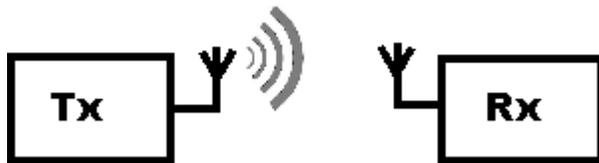
Fig.1 SISO - Single Input Single Output
