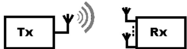
Fig. 2 SIMO- Single Input Multiple Output
