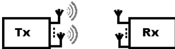
Fig.4 MIMO - Multiple Input Multiple Output
