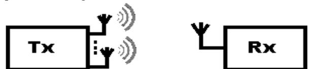
Fig. 3 MISO - Multiple Input Single Output
