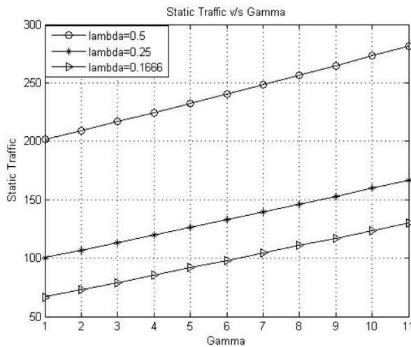
Figure-7 Static Traffic v/s Gamma for  $T_{RTP}=0.015$ s
